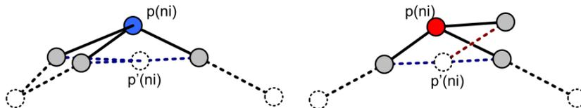
**Fig. 5.** Classification of nodes to be junctions or not. Left: edges to the projected node position  $p'(n_i)$  are all placed on a line (within a threshold), therefore  $n_i$  is not a junction. Right: edges do not form a line (red edge), therefore in this case  $n_i$  is a junction.
